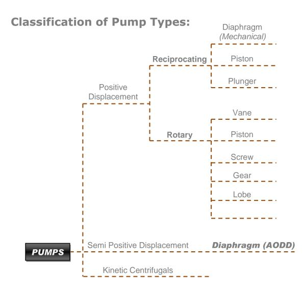
Although the AODD pump is a displacement type, it is actually a hybrid and defies strict classification. While its pressure versus capacity characteristics resemble those of a centrifugal pump, it is best defined as a Sealless, non (or semi) positive displacement pump. The pumping principle provides 100% efficiency at zero flow.
